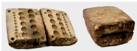
Fig. 17: Bivalve mold for casting projectiles of various diameters. The Carlists must have used similar molds to manufacture their bronze projectiles. Photograph by Ulrike, with authorization.
