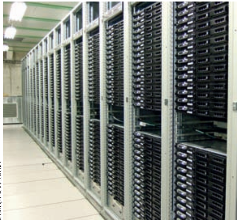
Figure 1. A rack of the Trigger and Data Acquisition System (TDAQ) of the ATLAS experiment at the LHC at CERN (Geneva).
